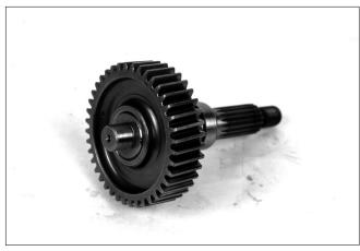
Check the countershaft for wear or damage.
