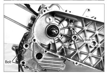
Loosen the seven R/L crank case setting bolts.
