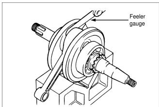
Check the vertical shaft play of the connecting rod big end from the X and Y direction.
