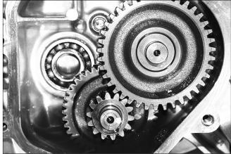
Remove the drive shaft from the transmission cover by using a hydraulic press.
