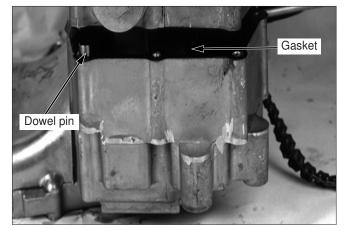
Assemble the R. crank case to the L. crank case.
