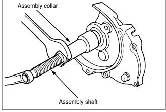
Install the final shaft and counter gear on the L. crank case.
