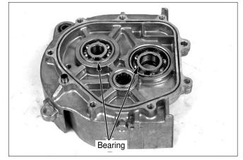
Use special tools to push in the bearing into the case.
